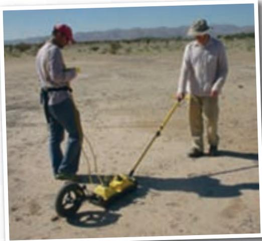
Employing Ground Penetrating Radar to detect buried falaj channels.
